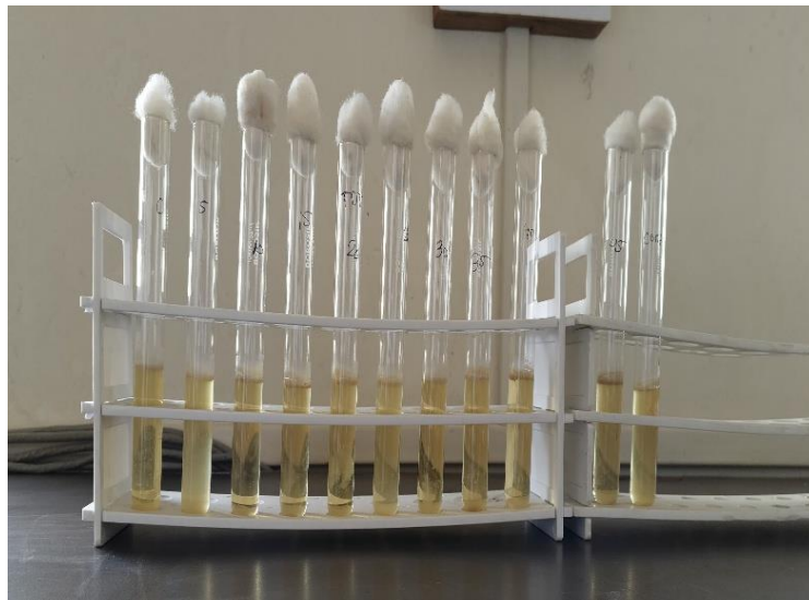
Figure 2: Tubes after incubation in Thermal death time experiment
